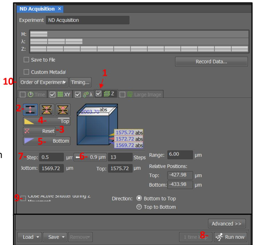
Figure 13: Z-Stack Acquisition-Top and Bottom
