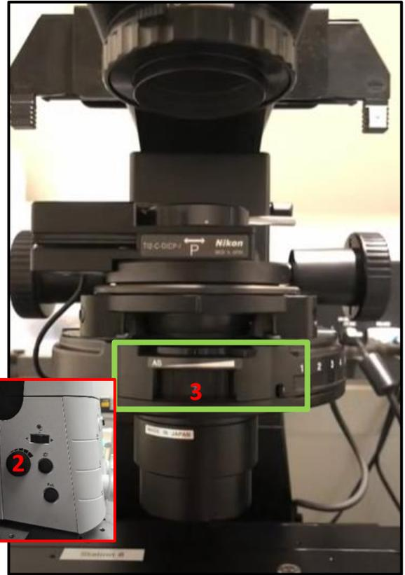
Figure 20: Köhler Illumination Aperture Diaphragm Adjustment
