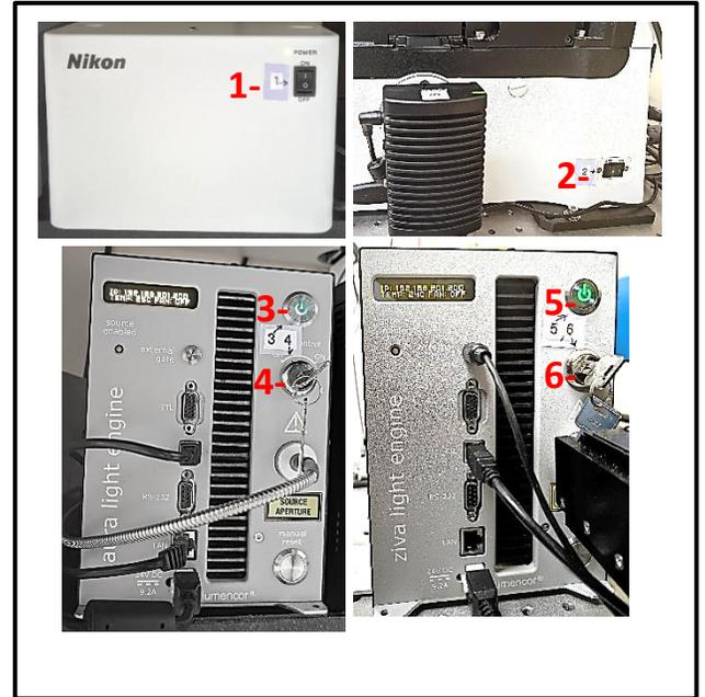
Figure 2: Turn on Microscope Stand & Illumination
