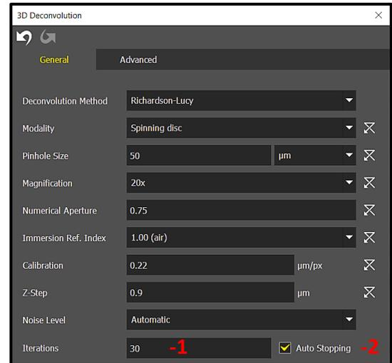
Figure 29: Richardson-Lucy Deconvolution
